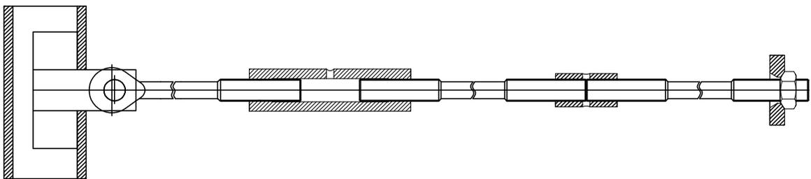
Alternative concrete connection option permitting rotational movement in all directions.
