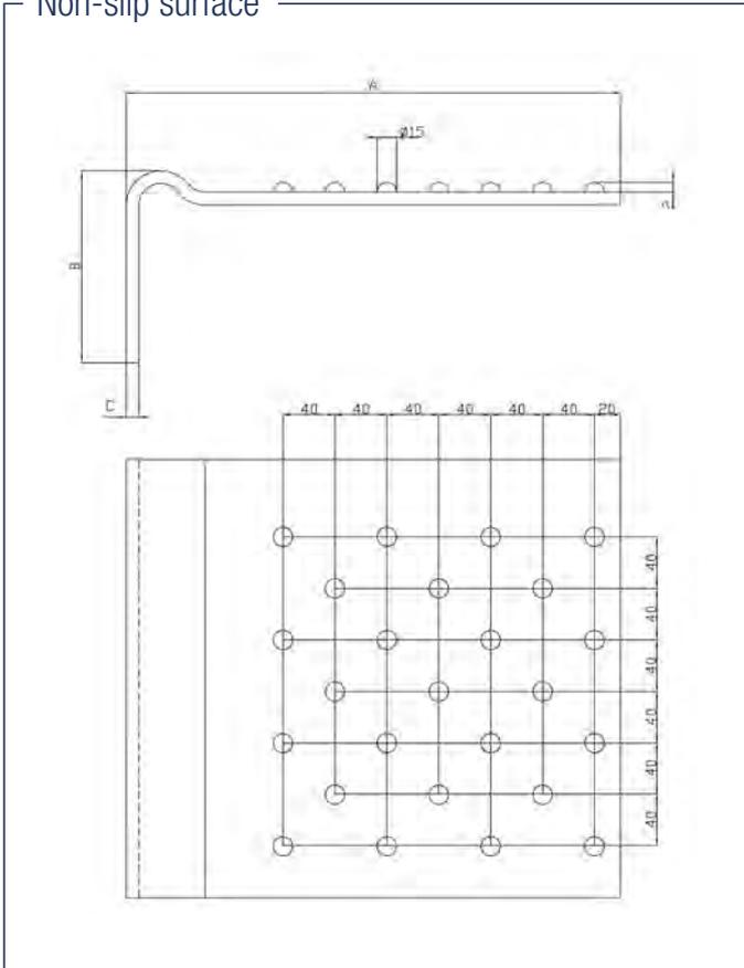
Ladder recesses for sheet pile wall cappings
