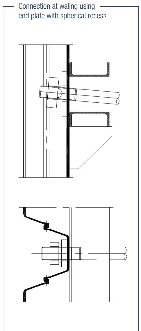
**When settlement is expected, the anchor connection should be hinged and allow movement in the vertical direction in order to avoid the associated bending stresses at the threaded joints. To allow movement, a rocker plate, end plate with spherical recess or threaded rocker plate is normally used.**
