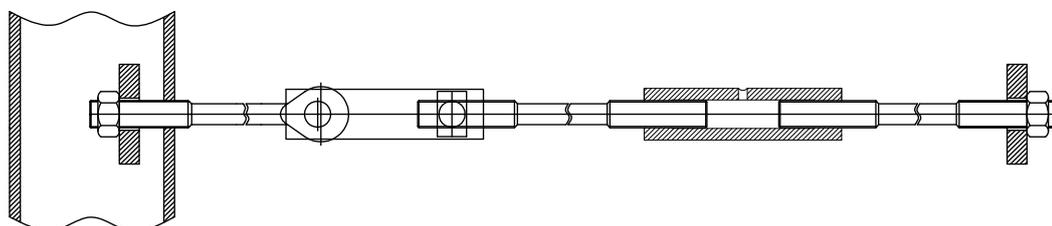
Typical option for anchors connected to tubular piles.
