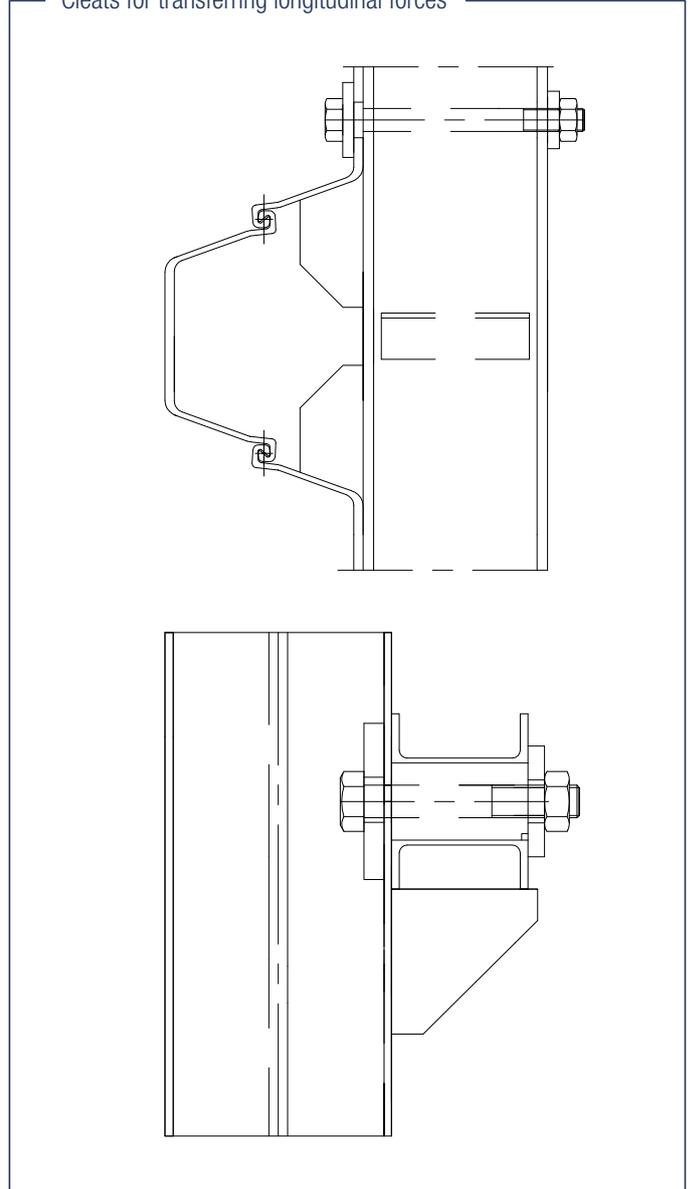
Typical connection to anchor wall
