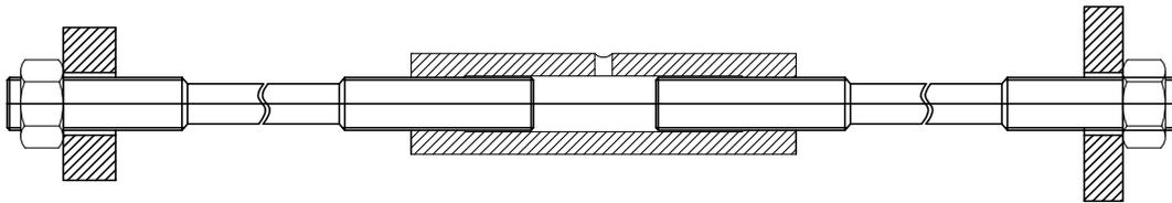
Anchorage for combined sheet piling with tubular piles.
